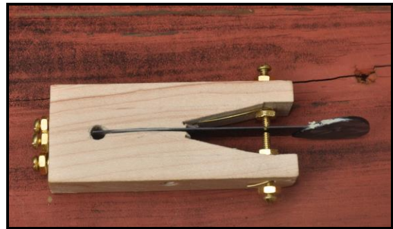
A single hardwood block and some brass machine hardware will also work FB!
