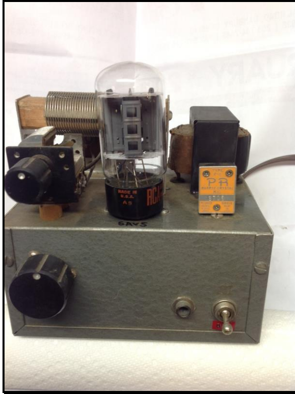
My first 5-watt crystal controlled transmitter – homebrew of course. Built by WA1FSU, now N1AOB
