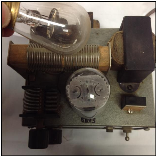
Tuning for maximum smoke (uum...brightness) using a neon bulb
