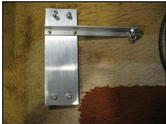
Custom designed and fabricated bracket for replacement fan dipole center support.
