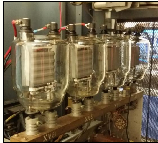
A robust pair of 833's modulating a second pair of 833's in the power amplifier.
