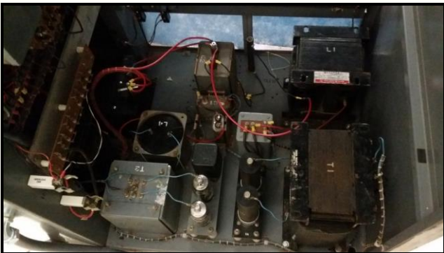
The plate voltage, modulation, and bias supply transformers and filter capacitors are attached to the bottom of the cabinet.
