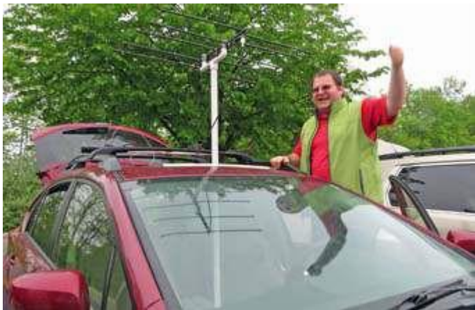
David KB1LTW adjusts his sunroof-mounted log-periodic by Elk Antennas shortly before the hunt.
