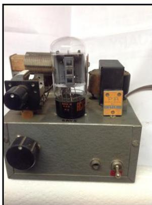
My first rig was a home brew one tube 15-watt transmitter for 80 meter CW only. I used a light bulb to tune for maximum output power. Still have it!
