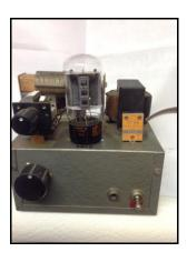
My first rig was a home brew one tube 15-watt transmitter for 80 meter CW only. I used a light bulb to tune for maximum output power. Still have it!
