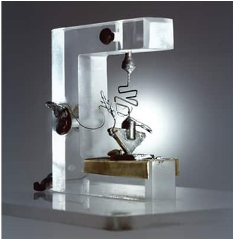
Figure 7: The Point Contact Transistor (Reused with permission of Nokia Corporation)
