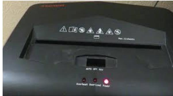
Some shredders also have a photo sensor to control the motor, and if it gets dusty will allow the motor to run continuously. A plastic drinking straw can be used to blow air into the input slot and clean the sensor, allowing the motor to shut off after the paper has been shredded.
