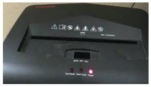
Some shredders also have a photo sensor to control the motor, and if it gets dusty will allow the motor to run continuously. A plastic drinking straw can be used to blow air into the input slot and clean the sensor, allowing the motor to shut off after the paper has been shredded.
