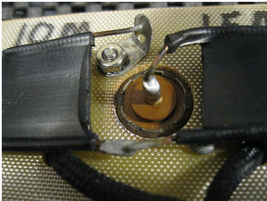
MFJ ladder line center insulator and ladder line connection to SO-239 Photos: W1QK
