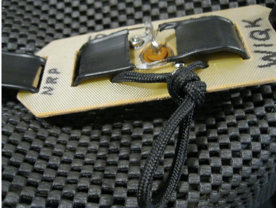
Detail of MFJ - Model 16F01 Ladder Line Center insulator and rope knot used for hanging inverted Vee from support.
