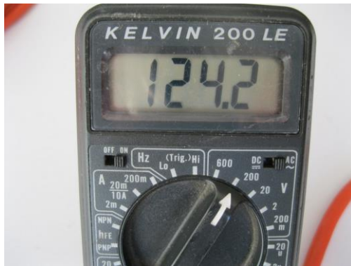
Measured unloaded generator AC output voltage
