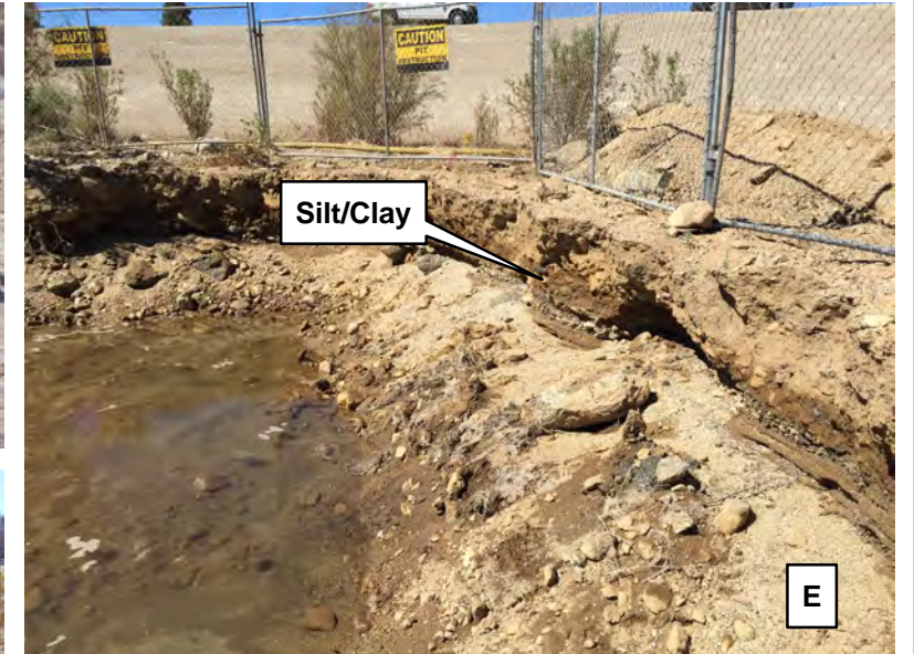
A. 4" fire hose / YVWD fire hydrant in background B. Post-excitation / fencing setup (Day 1) C. Test in progress (Day 3) D. Test in progress (Day 4) E. Post-testing - hard silt/clay layer shown in upper 3 feet
