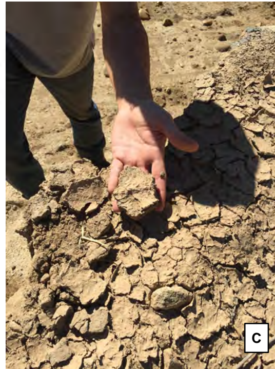
A. 4" fire hose / YVWD fire hydrant in background B. Bermed (background) and Excavated Basin (foreground) C. Fine silt/clay on ground surface D. Post-excavation and plastic sheeting bermed basin E. Testing in progress (Day 1) F. Leaked recharge water east of test basin (Day 6)
