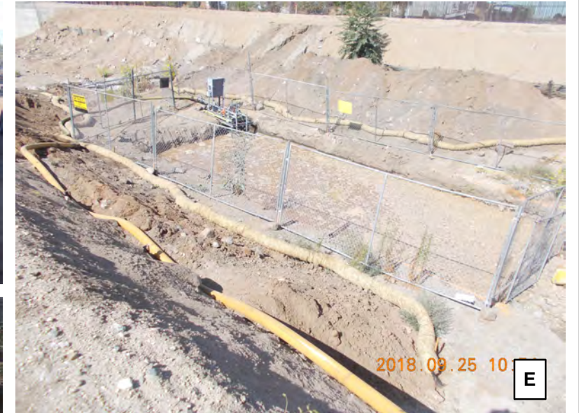
A. YVWD hydrant at 10th Street and 4" fire hose B. 4" fire hose along northern channel bank west of 10th Street C. Excavated basin, fencing, and soil stockpile D. Initial test basin filling (Day 1) E. Falling head test in progress view from south (Day 2)
