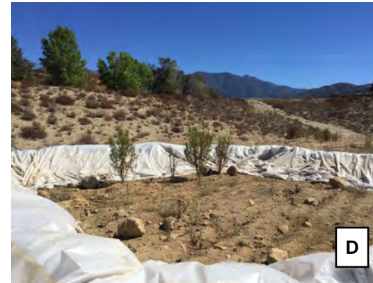
A. 4" fire hose / YVWD fire hydrant in background B. Bermed (background) and Excavated Basin (foreground) C. Fine silt/clay on ground surface D. Post-excavation and plastic sheeting bermed basin E. Testing in progress (Day 1) F. Leaked recharge water east of test basin (Day 6)
