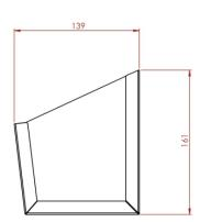
Height: 161mm Width: 193mm Depth: 139mm Weight: 1Kg Capacity: x1 5 Ltr Bottle
