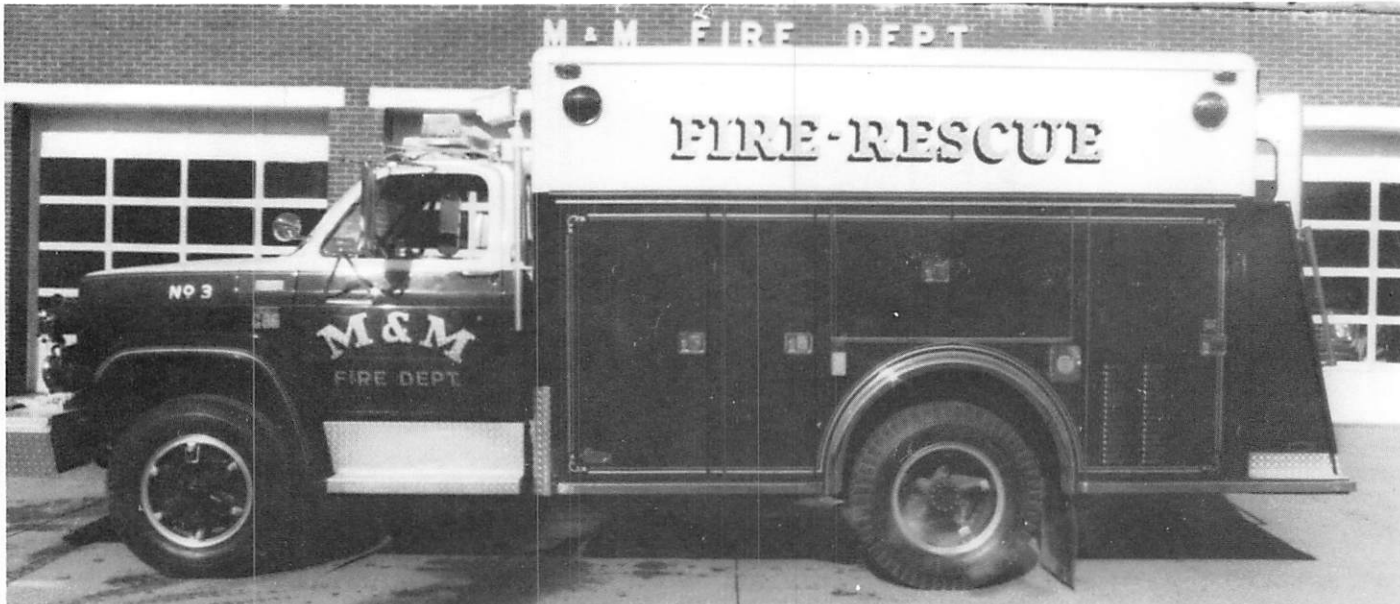
1978 Pierce heavy duty fire/rescue unit designed by M&M Fire Dept. for multi-purpose utilization. Used on all fires and rescues. Has a 750 GPM pump, carries a Hurst tool and other crash rescue equipment. Designed for manpower to ride in out of the weather.
