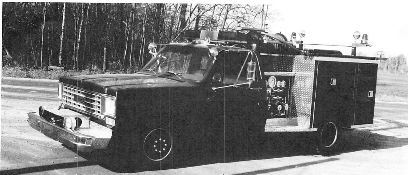
1978 Pierce 400 GPM Mini Pumping apparatus mounted on a Chevrolet Chassis, K-30, four-wheel drive with 250 gal. booster tank, booster reel of 200' of 1" hose, PTO front winch, capable of discharging 700 GPM from exterior water source. Replaced grass truck 2 in 1980.
