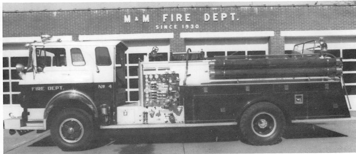
1970, 1000 GPM triple-combination pumping apparatus, the first apparatus in southeastern Ohio with a preconnected, 2½" Blitz line. The first 1000 GPM pumper delivered to a Volunteer Fire Dept. in Southeastern Ohio.
