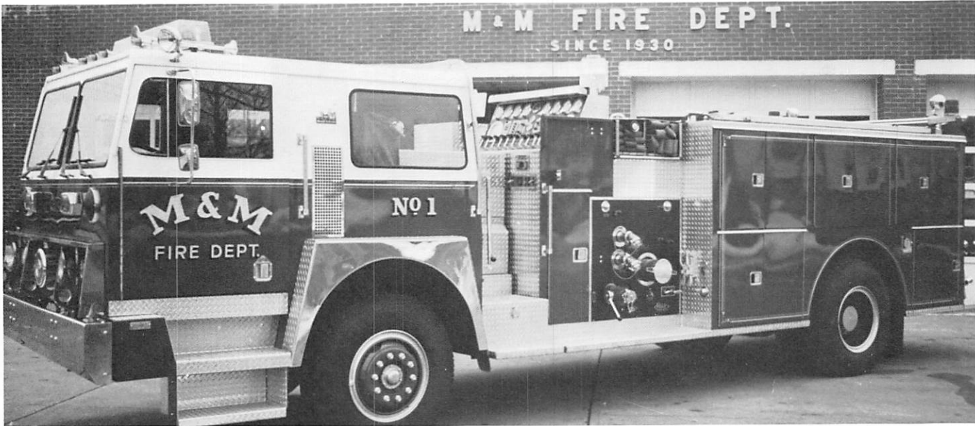
1977 Pierce Custom, 1500 GPM triple-combination pumping apparatus, designed exclusively for the M&M Fire Dept. Equipped with many of the latest innovations in the fire service. The first pumper of this size in Southeastern Ohio. Instrumental in obtaining Class 5 insurance rating.
