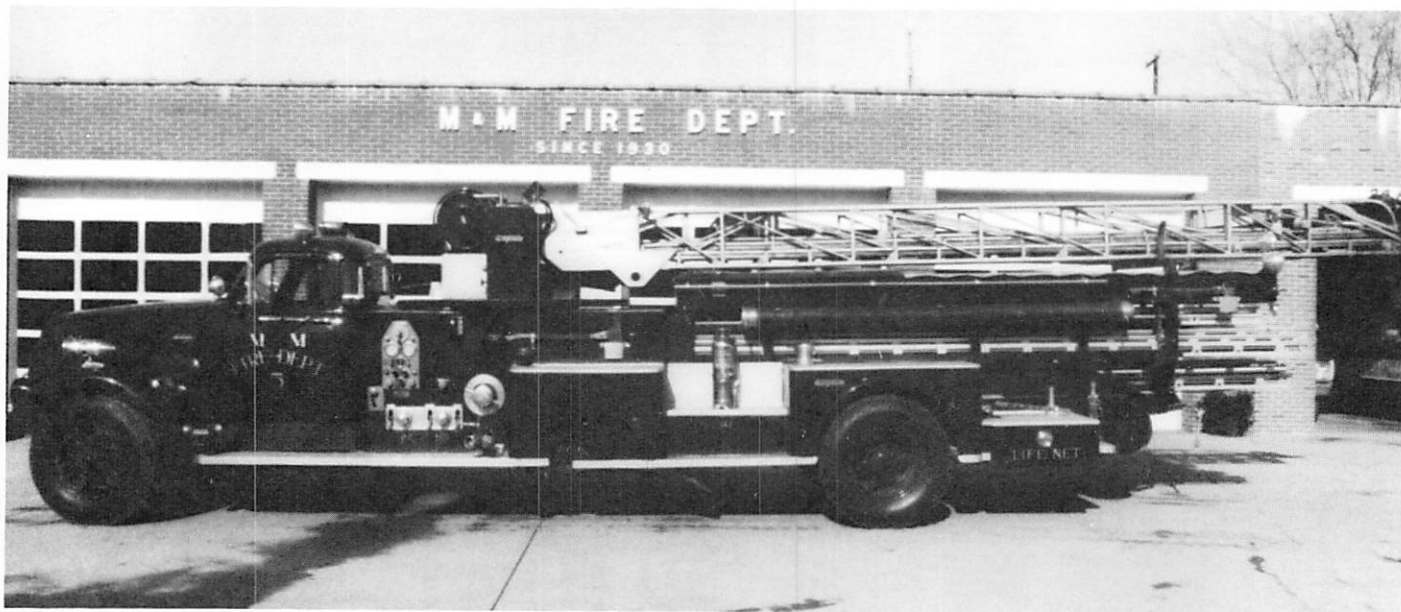
1967 Seagrave Quint ladder/pumper apparatus. Delivery of this apparatus resulted in the two Villages going from Class 8 rating to Class 6 insurance rating. 65', three-section hydraulic operated aerial ladder, 198' of ground ladders, ladder pipe with fog head.
