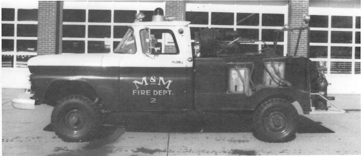
1960 Four-wheel drive utilized for off the highway use, such as grass fires, wood fires, etc. Carries 200 gallon of water, portable pump, and miscellaneous equipment. Designed and built by the M&M Fire Dept.
