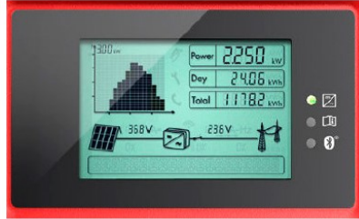
LED Green - Indicating correct operation of inverter
