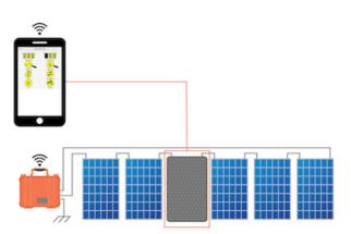
Figure 4: In the illustration we see the general approach to the module test. First a reference spectrum is recorded without any modules shading. Individual solar module are then shaded one by one, while the main measurement parameters are recorded.
