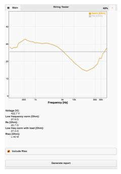
Connect the instrument to the PV string and press the Measure button to collect a spectrum. The measurement will take 30-60 seconds. In the example shown to the right,  $R_s$  is 16.9  $\Omega$  as is the low frequency norm at a voltage of close to 410V, which indicate a healthy string of 12 x 250 W modules with a decent sun irradiation. With a higher irradiation Rs could go as low as 10  $\Omega$ .
