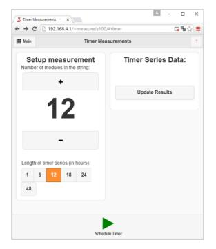
The number of PV modules "N" must be adjusted using the + and - buttons. Select the duration/length of the timer test using the buttons: a ground fault test will be conducted every 15 minutes during the duration of the test. The Schedule Timer button will start the test when pressed. The WiFi antenna will close down during test
