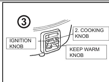
6. To ignite main burner push **2. COOKING** knob down. Check main burner ignition by viewing through the 6 view holes.
