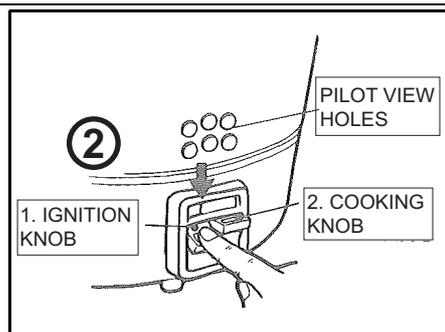
3. Release **1. IGNITION** knob, check that the pilot is lit by looking through the six pilot view holes. **1. IGNITION** knob will return and **KEEP WARM** knob will stay pushed down.
