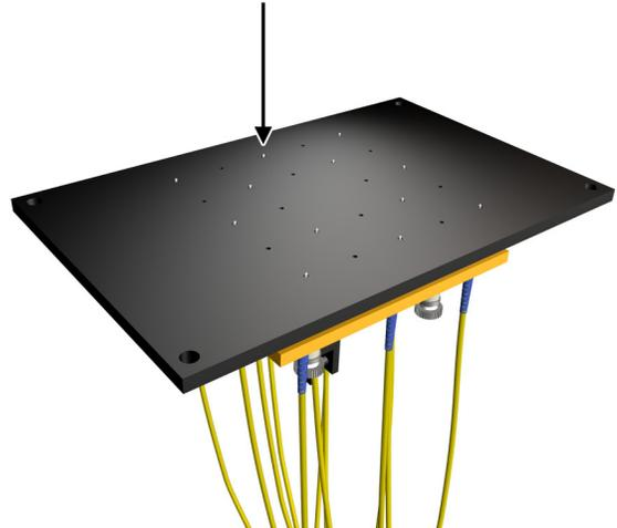
4) Lift up plate and press on the ferrules, checking to make sure the connectors have spring action and none are locked in place. Place the **Fixture Plate** back onto the **Fixture Holder**.
