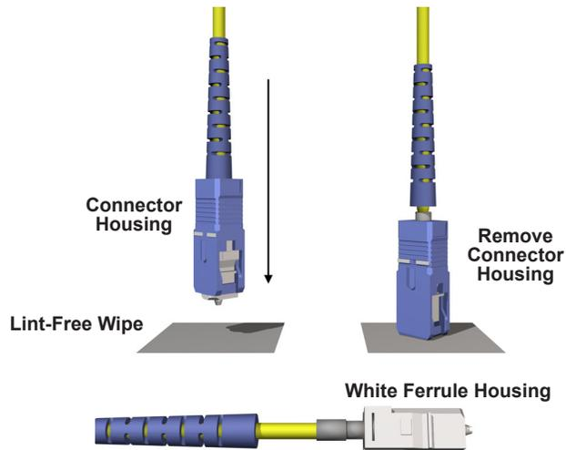
**It is important that the SC Connector is polished prior to assembly. Make sure the outer housing is off and boots are pulled back.**
