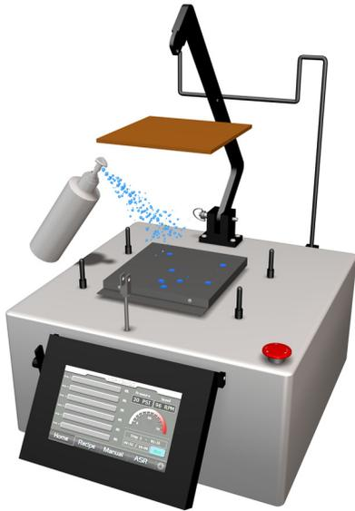
3) Spray a very small amount of distilled water onto the surface of the **Base Plate**.
