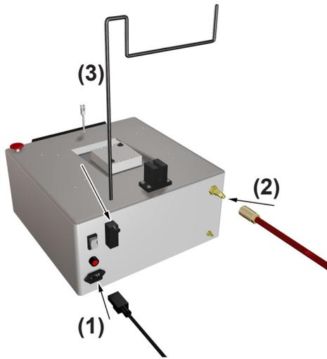
**1)** Plug in **Power Cord(1)** into the back of the **ACP 24/96**. Before plugging in **Air Hose(2)**, make sure the air pressure is set to zero to avoid damaging internal components and the maximum air pressure does not exceed 100 PSI. Plug **Power Cord** into your power source (with surge protection) and the **Air Hose** into your air source. Insert **Cable Tree (3)**. Do not tighten.
