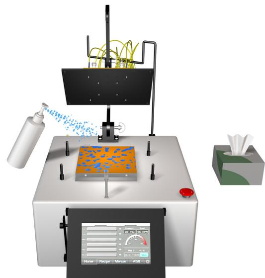
6) Lift the arm to expose the **Rubber Pad**. Spray distilled water onto the Rubber Pad and use a **Lint-Free Optical Wipe** to clean the surface.
