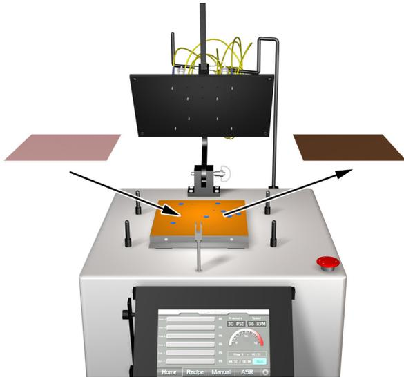
**9a)** Replace the **6um Diamond Film** with the **3um Diamond Film**.
