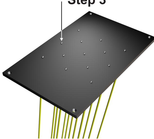
**3)** Lift up plate and press on the ferrules, checking to make sure the connectors have spring action and none are locked in place. Place the **Fixture Plate** back onto the **Fixture Holder**.
