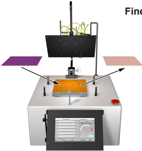
**10a)** Replace the **3um Diamond Film** with the **1um Diamond Film**.
