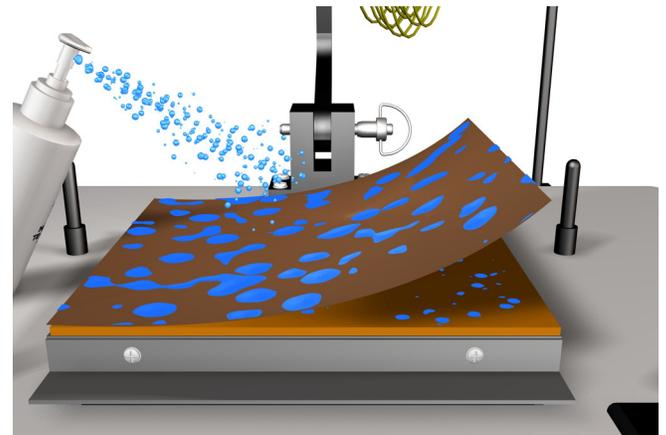
**8b)** Place the **6 um Diamond film** with the smooth shiny side down on the rubber pad.
