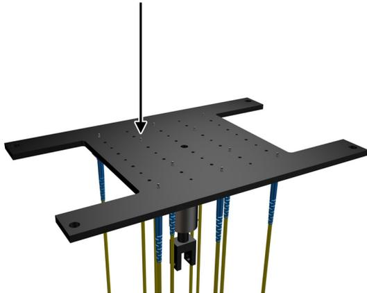
**3)** Lift up plate and carefully press on the ferrules, checking to make sure the connectors have spring action and none are locked in place. Pressing too hard may cause a connector to pop free. Place the Fixture Plate back onto the Fixture Holder.
