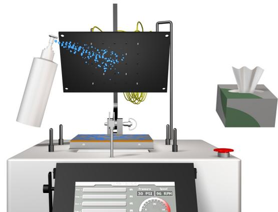
**7d)** After polishing has finished, remove the small push-pull pin and lift the polishing plate.
