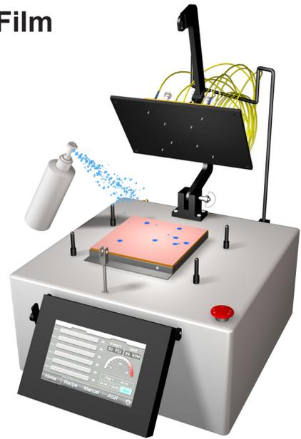
**9b)** Spray distilled water onto the surface of the film and wipe clean using lint-free wipes. This procedure will ensure a clean working surface and remove any large air bubbles.
