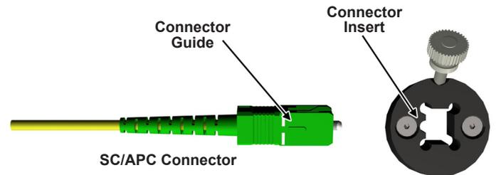
Insert the **SC/APC Connectors** into the **Fixture Plate**. Note that the guide on the top of the connector slides into a slot located in the **Connector Insert** of the **Fixture Plate**. Make sure the connector has been pushed to the bottom of the **Connector Insert**.
