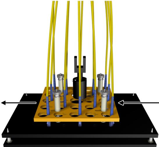
3) Loosen the **Locking Plate** and slide it over the connectors. Then retighten the **Locking Plate**. Tighten nuts diagonally.
