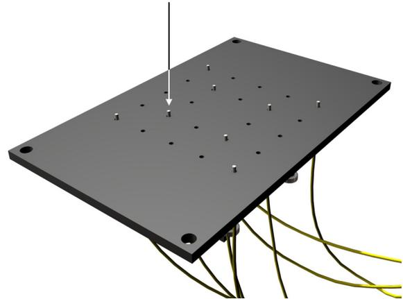
**4)** Lift up plate and press on the ferrules, checking to make sure the connectors have spring action and none are locked in place. Place the **Fixture Plate** back onto the **Fixture Holder**.
