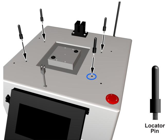
**2)** Insert the **Fixture Plate Locator Pins**. The inner holes are for MCP 24 Fixture Plates. The outer holes are for MCP 48 Fixture Plates.
