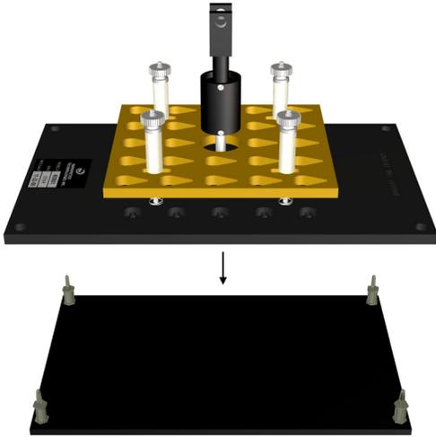
**1)** Make sure the **Fixture Plate** is free of particles. Place the **Polishing Fixture** on the **Fixture Holder**.
