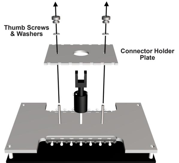
2) Remove the **Thumb Screws & Washers**. Lift and remove the .
