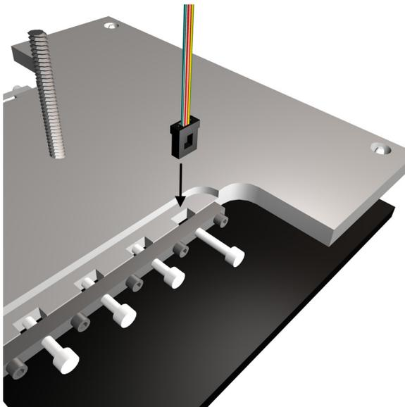
3) Loosen the **Nylon Screws** that will hold the connectors.
