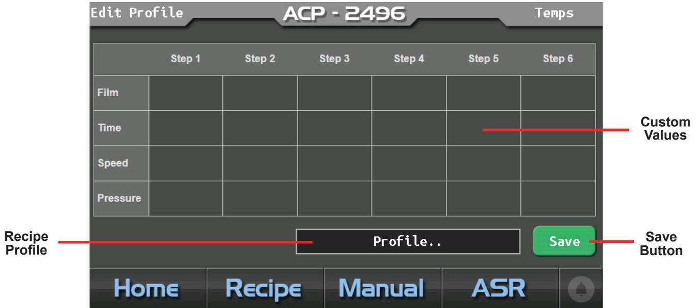
Use the Edit Recipe function to create custom polishing recipes or make adjustments to existing recipes. Press an empty box under each step to enter a custom configuration.
