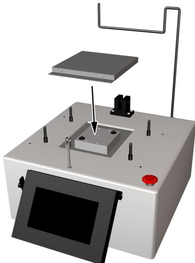
**3)** Set the **Base Plate** on the **Interface Plate**. Make sure both surfaces are clean. Use the guide holes on the **Base Plate** to line up with the **Interface Plate**.
