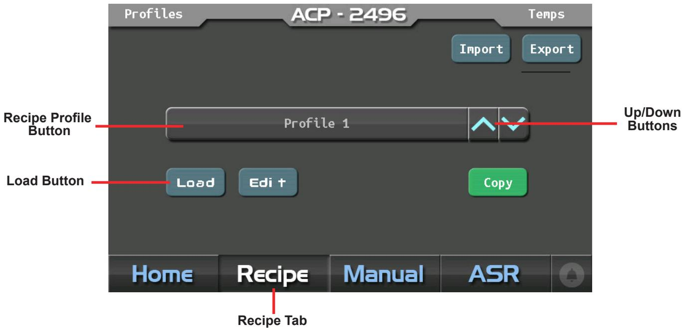
**1)** Press the **Recipe Tab** on the bottom of the screen. Press the **Profile Button** to select a **Fixture Plate**. Use the **Up/Down Arrows** to find the fixture plate. With the fixture plate selected, press the **Load Button**. Return to the home page by pressing the **Home Tab**.
