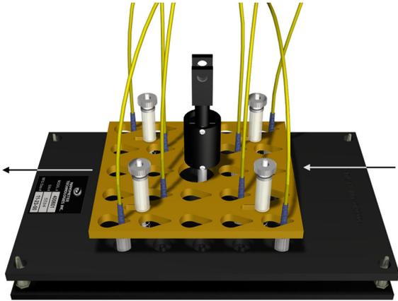
**3)** Loosen the **Locking Plate** and slide it over the connectors, then re-tighten the **Locking Plate**. Tighten nuts diagonally.
