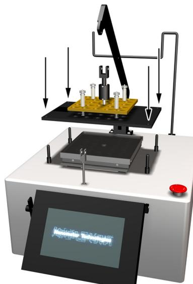
4) Place the **Fixture Plate** on the ACP 24. Make sure the **Fixture Plate** fits onto the 4 locator pins.
