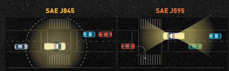
SAE J845 is for omnidirectional or 360-degrees of warning light. Commonly used to clear traffic. SAE J595 is for directional flashing optical warning lights. Commonly used to direct traffic away from a work zone area.
