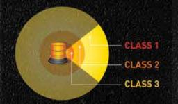
SAE relies on Candela to create class rankings. SAE J595 and SAE J845 are standards that refer to the functionality (purpose) of the light source on a vehicle. Within the SAE J845 and SAE J595 specification are Class 1-2-3 rankings which measure the light intensity at specific data points and candela intensity to determine the Class level of the warning device.
