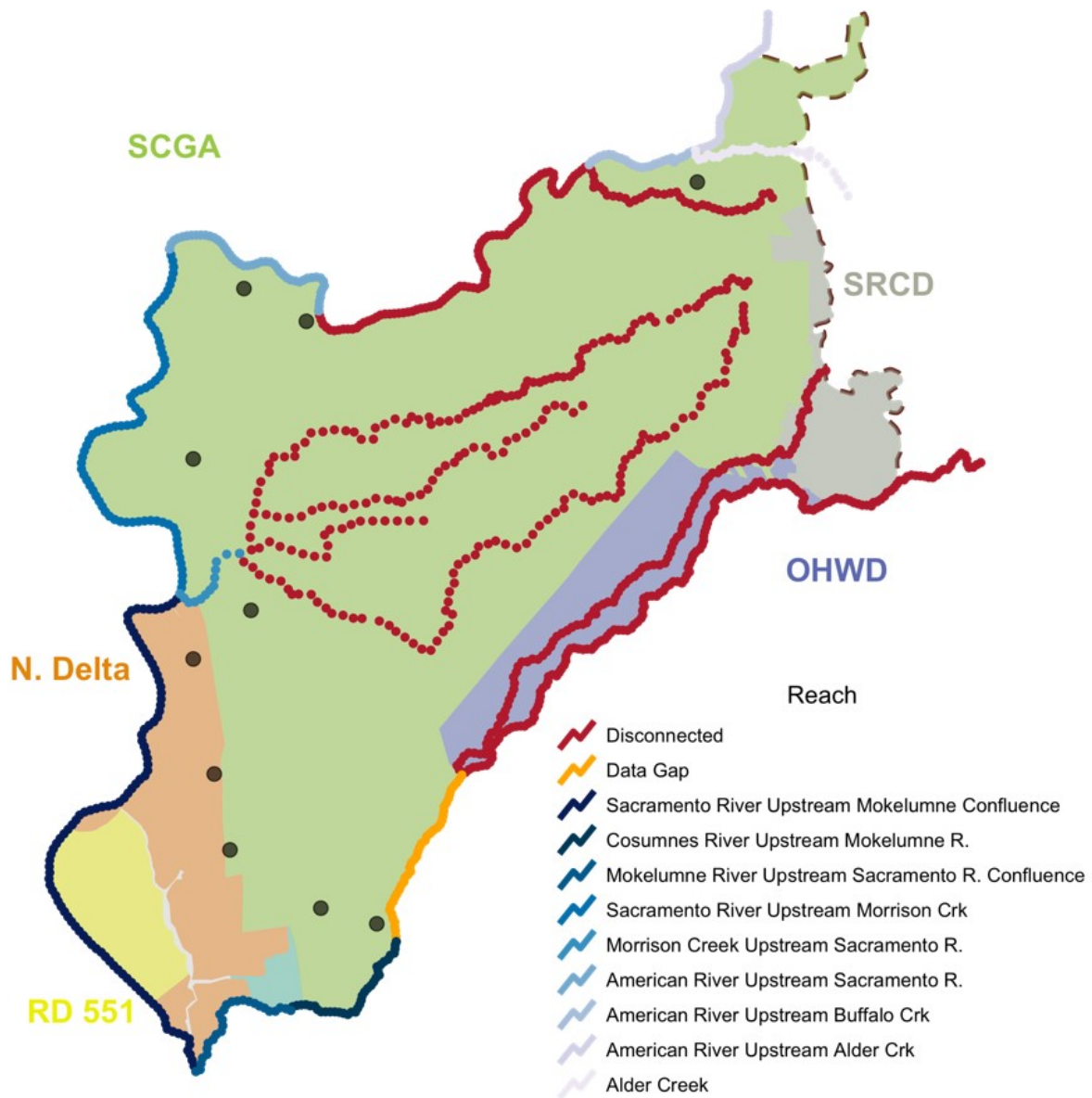
Figure 3-11: Probable ISW reaches by name, Probable Disconnected reaches, and GSAs in the Basin. Classification of reaches follows the methodology summarized in Section 3.3.1.2, Figure 3-8, and Appendix 3-A. Grey points indicate the locations of ISW RMPs in the GSP monitoring network.
