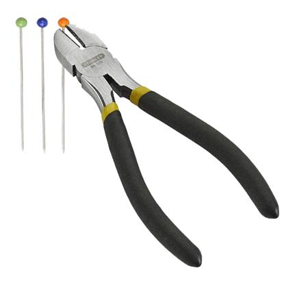
Cut the head off a 1 1/2" sewing pin at the head. Cut another pin off about 1/4" shorter than the first pin. Cut another pin off about 1/2" shorter than the first pin.
