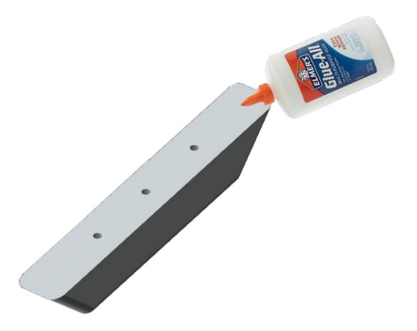
Place a moderate bead of white clue around the holes on the bottom of the base and work the glue into the holes. Then, wipe off the residual glue from the bottom.
