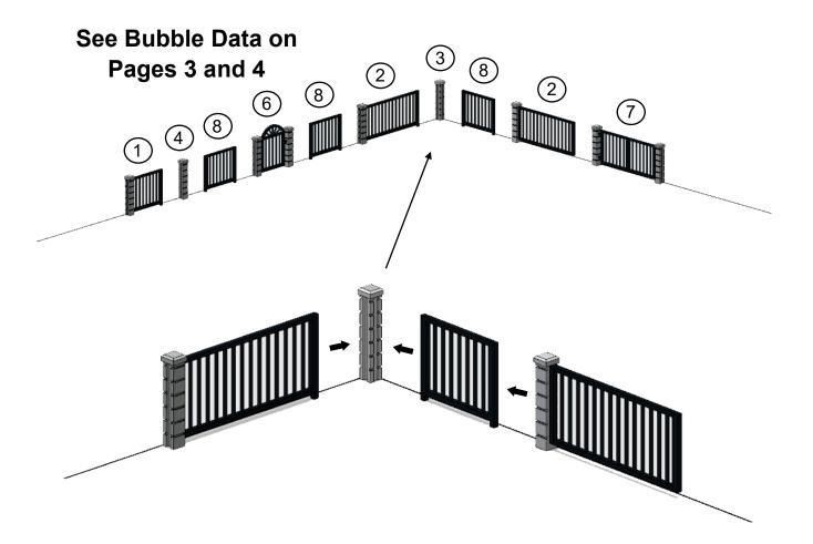
Draw perpendicular construction lines on your layout at the point where you wish to start installing the fence. The lines will help keep the wall straight during installation.
