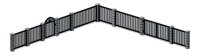
Each piece of my interconnecting Rod Iron Fence system has an end grove and/or tongue for easy and accurate installation.
