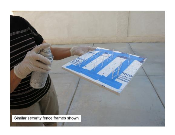
Put a disposable glove on your hand that will be holding your work so you will not accidently paint your hand too. Step outside or wherever you spray paint and give your fence parts a good coat of aluminum colored paint that bonds with plastic. I use Rust-oleum 2x Ultra Cover paint. Set your painted work aside and let it dry 20-30 minutes. Now you can prepare the next piece of insulation and add more fence parts to paint.
