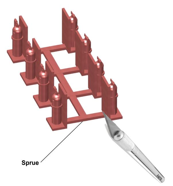
After the paint dries, use an Exacto Knife or Utility Knife to cut away the joining strip (called "sprues). The sprues are used to make the extinguishers an integral model during printing, similar to the old injection plastic models. This keeps the printing cost much lower.
