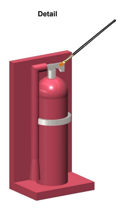
Use a small paint brush and carefully paint the valve and securing strap silver or aluminum.
