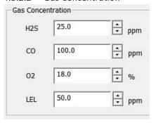
This field allows you to enter the gas concentration(s) of the test gas cylinder installed in the Bump-Calibration Station. This is necessary for proper testing and calibration of PM100 monitors. There are fields available for H2S, CO, O2, and LEL.
