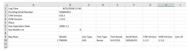
Each PM100 monitor that is tested using the Bump-Calibration Station will generate its own log file. The log file shows entries for events, bump tests, and calibration tests. The image below shows the information in a sample log file.
