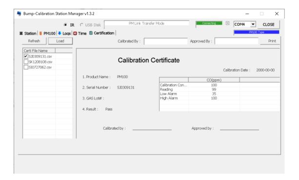
The certification tab is used to create a physical certificate upon completion of calibration. A printed record should be made and kept every time a unit is calibrated.
