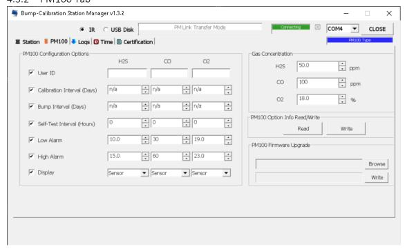
The Bump-Calibration Station and Bump-Calibration Station Manager software can be used to quickly make configuration changes for multiple PM100 detectors. The PM100 tab in the Bump-Calibration Station Manager software shows the available configuration options for PM100 devices. All configuration settings can be set to be simultaneously updated during each bump test or calibration (see Section 5.3.1.2 Enable/Disable Function).
