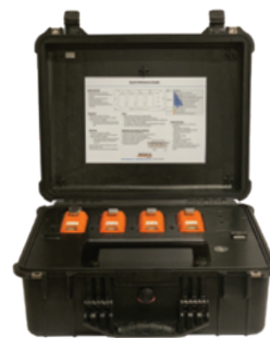
Bump/Cal Test Station
