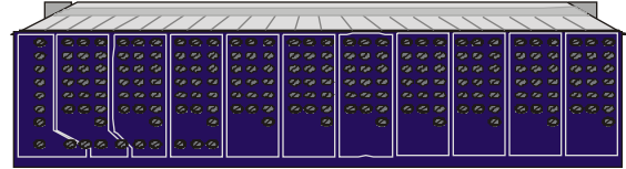
CS-60 REAR VIEW SHOWING BACKPLANE AND 19" RACK FOR 60 ZONES LOOPS AND LED TERMINATIONS
