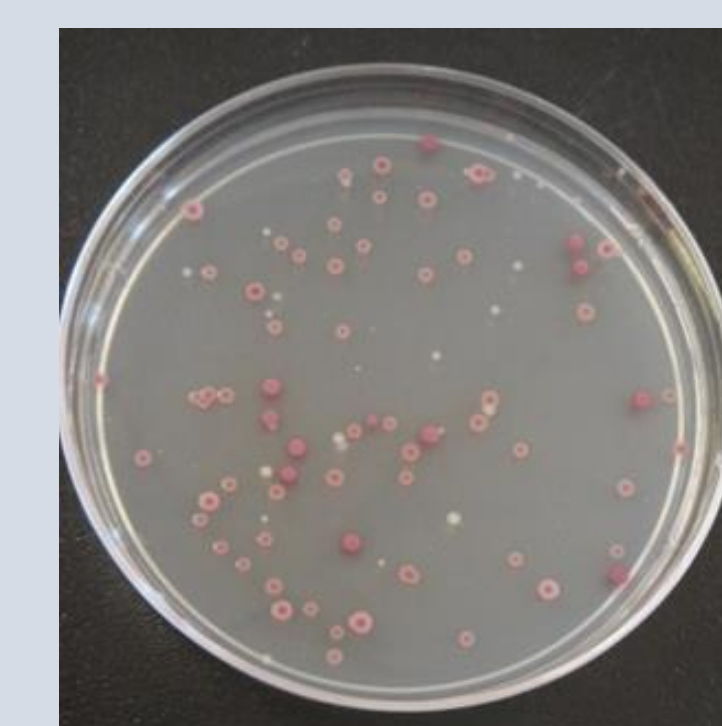
Filter water bacterial analysis Chromogenic medium
