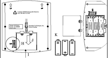
This unit comes equipped with 3 AA, 1800 mAh NiMH rechargeable batteries. Turn the switch (H) to OFF position and remove the screw (I) and slide Battery Cap (J) down. New batteries can now be installed according to their proper orientation (K). *Note: Batteries should not be replaced unless results have decreased dramatically. Old batteries should be recycled properly.*
