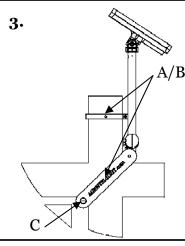
3. Locking the Unit Security is a critical component found in the AGENTSLIGHT<sup>™</sup>. Insert lock at the end of Pin (C). The Support Ring has also been equipped with a stopper to prevent any tampering. The Support Ring (A) and Lock Arms (B) have screw holes for optional security.
