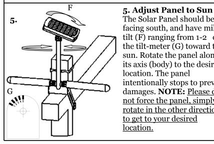
The Solar Panel should be facing south, and have mild tilt (F) ranging from 1-2 on the tilt-meter (G) toward the sun. Rotate the panel along its axis (body) to the desired location. The panel intentionally stops to prevent
