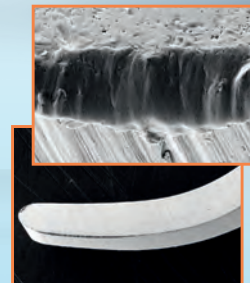
Cutting edge of an typical non-coated curette and the magnification of the edge after the test.
