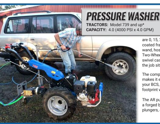
The Pressure Washer comes with a 50' hose, 36" pistol-style wand, and five tips for variable pressure output (angles
