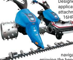
Designed for commercial slope mowing applications and oriented for front-mount attachments only, Model 660 features a 16HP twin cylinder Vanguard engine to provide both the power and engine oil lubrication needed for slopes up to 30 degrees. Hydraulically-activated, individual clutch-brake mechanisms allow operators to effortlessly
