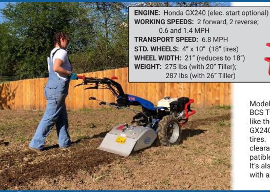
Model 722 is the most popular straight-axle BCS Two-Wheel Tractor model. Built much like the 718, but with a more powerful Honda GX240 engine and larger standard wheels/ tires. The extra power and increased ground clearance greatly expand the range of compatible attachments available for Model 722. It's also the smallest tractor model offered with an electric start option.
