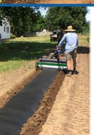
With an updated design, the Plastic Mulch Layer now supports both 36" & 48" plastic rolls. It will flat-lay 36" plastic, leaving approx. 26" exposed. It will also flat-lay 48" rolls, leaving approx. 38" exposed. Raised beds
