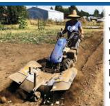
The Power Ridger is unique for a soilworking attachment as it is operated in front of the tractor. It leaves an open trench with ridges on either side, perfect for bulb or tuber planting. Soil discharge is controlled by the individually adjusted and extendable
