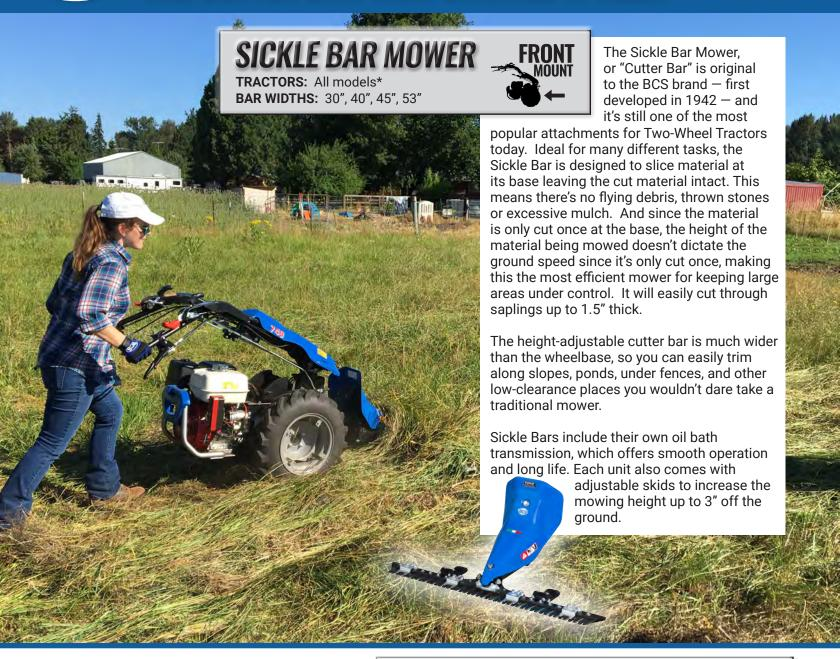
The BCS Dual Action Sickle Bar Mowers step it up a notch from their single-blade predecessors. This unique and fast sickle bar attachment mows using two moving blades, each moving in equal and opposite directions. The dual-action reduces vibration for the operator and enables the operator
