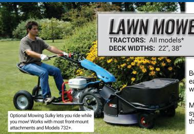
Save time, maintenance, and storage space by making your BCS tractor a manicured lawn mower, too! The BCS Lawn Mower outperforms most walk-behind mowers in the market with a steel deck and heat-treated steel gears running in oil bath.
