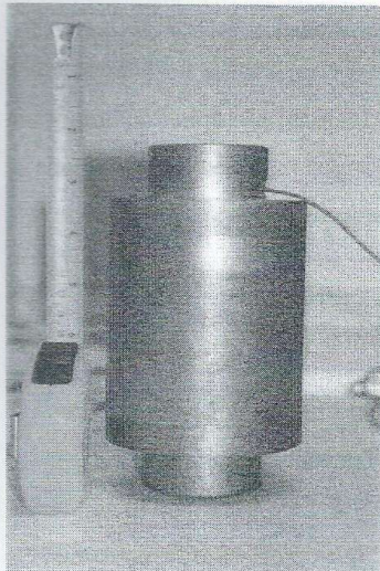
Figure 3.3a Eight kg weight used to simulate impacting knee of a dairy cow
