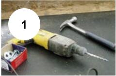
Tools needed: a hammer drill and a hammer. In most installations the mats may have to be shortened so you will also need a sharp knife and a chalk line. We recommend a low cost utility knife with "snap-off" blades. It is also helpful to use some kind of 2 inch spacer to ensure mats are always at least 2 inches apart.
