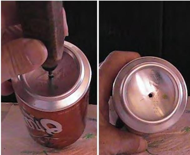
Cut the top off each can just above the bend where it narrows. You can either cut it off using a utility knife or punch a starting hole and cut the top away using scissors.
