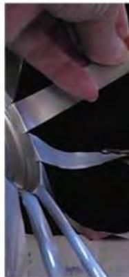
Repeat the process all the way around until all the spokes of one can are joined to the spokes of the other.
