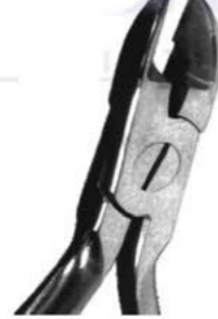
Hard wire cutter 13 cm / 5" 786-2109 Box Joint 786-2110 Screw Joint 786-2111 L-Key Joint For cutting orthodontic wires for fixed techniques any size. Cuts rectangular wire up to 0.56x0.71mm and round wire up to 0.51mm
