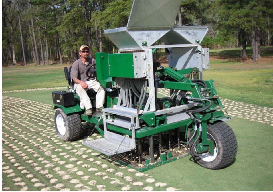
Drill & Fill Deep Drill Aerator & Backfill
