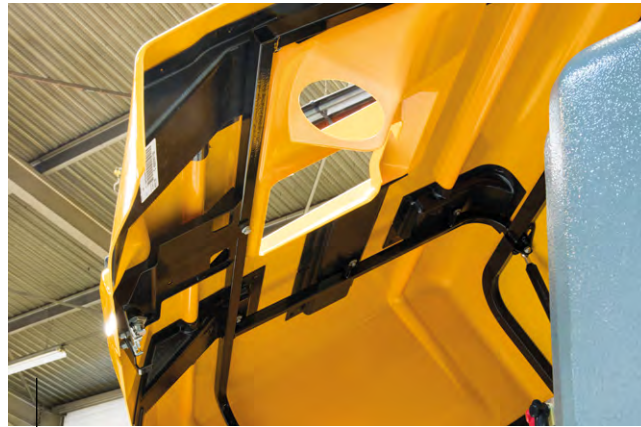
REINFORCED TURRET HOODS with metal support framework
