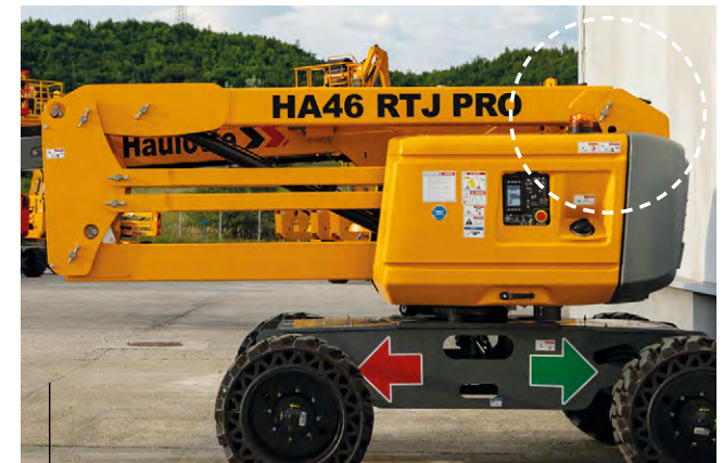
BOOM PROTECTED by the counterweight frame
