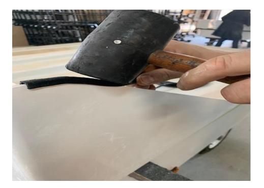
NOTE: Do not try to measure ahead and cut to size. Work your way around the entire lid to the other end...then cut to EXACT size. Again this is a *friction fit* and simple patience is required to gently force the bead into place in one piece
