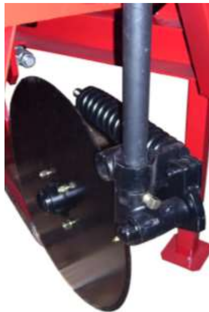
Figure 9: Completed Coultter Assembly
