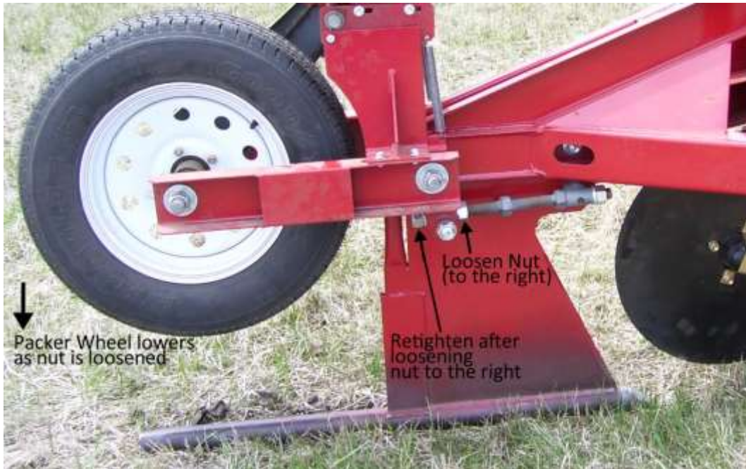
Figure 12: Packer Wheel Adjustment
