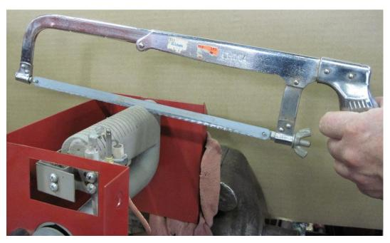
Figure 5: Servicing burner slots with hacksaw blade
