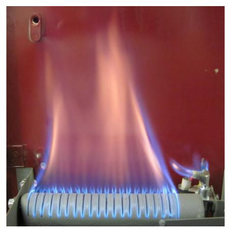
Figure 8: Burner with Insufficient Air
