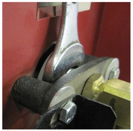
Figure 7: Adjusting the Locknut Holding Air Adjustment Disc in Place
