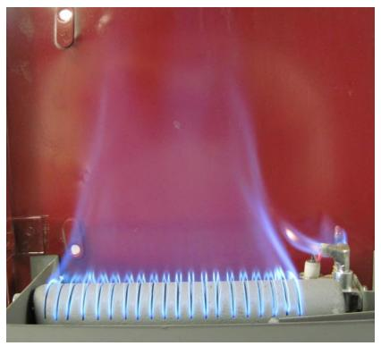
Figure 6: Correctly Adjusted Burner Flame
