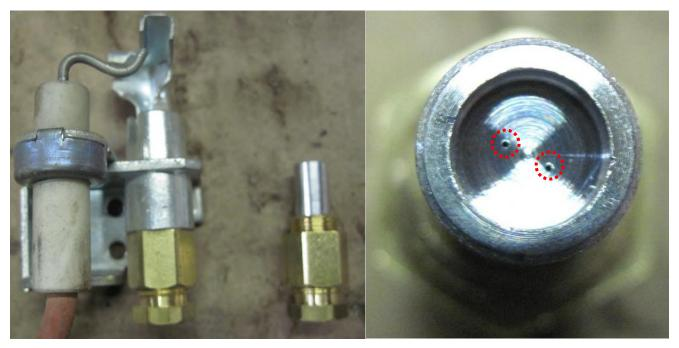
Figure 3: Pilot Light Orifice Mounted in Pilot Light Assembly (Left) Orifices, quantity 2, within Pilot Light (Right)
