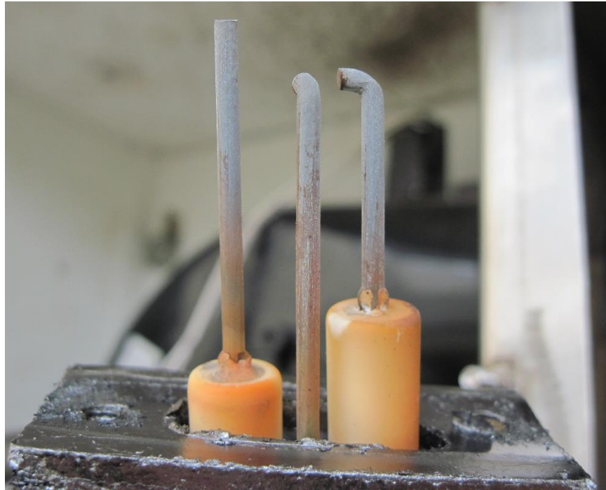
Figure 4: Uninstalled Electrode Assembly after 1 year of operation
