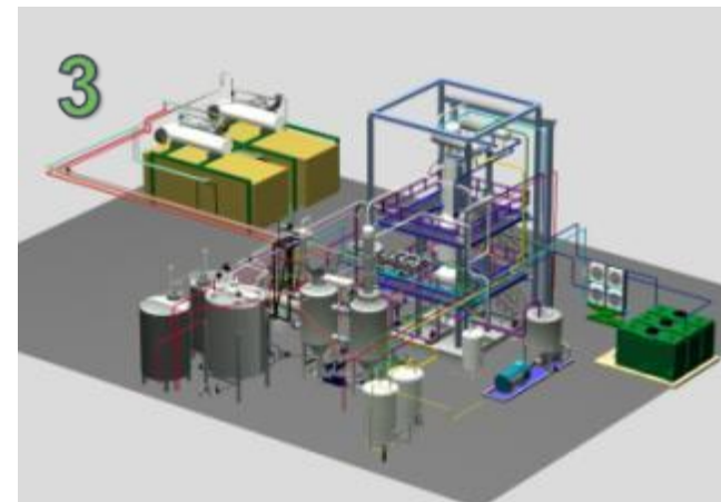
Alkat plant with link to diesel tanks
