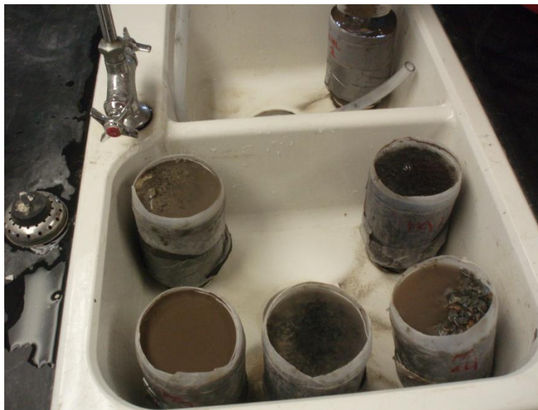
Figure 22: Surface materials in ½ gallon containers being loaded and draining in sink
