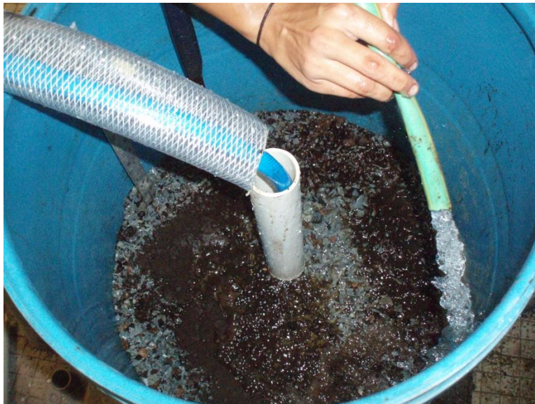
Figure 47: Washing loaded sediments into pores while pumping infiltrated water out through well pipe
