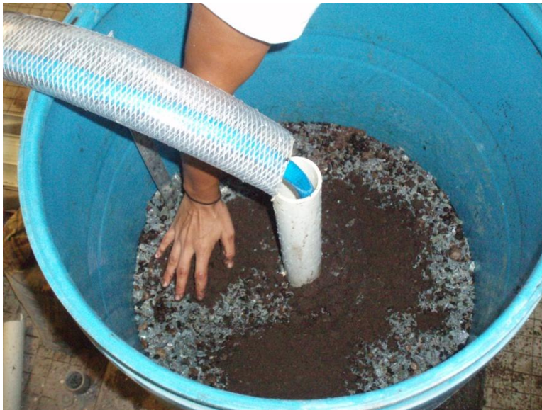
Figure 27: System barrel being loaded with sediments
