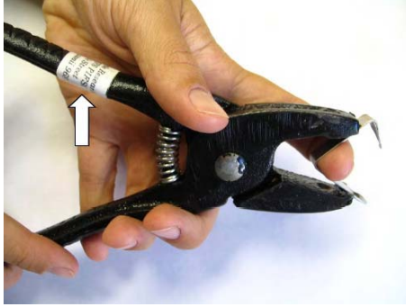
Figure 5.8: Loading a flipper tag into tag applicator. The arrow indicates which handle should be up.
