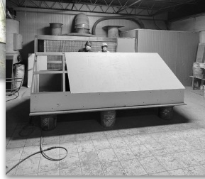
Image: Mold production for Ellie Tower podium by Petra Design
