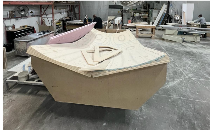
Image: Wooden mold for Mosque Dome
