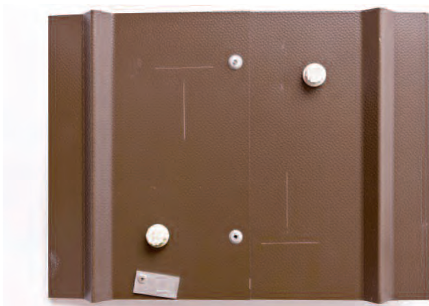
Figure 16. Colorcoat HPS200® with Galvalloy® metallic coating – 6 years exposure at coastal weathering site at Rye, England.
