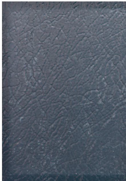
Figure 28. Anthracite standard leathergrain and Colorcoat HPS200 Ultra® after 2000 total hours in UVB test
