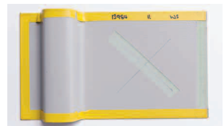
Figure 22. Test panel after Watersoak 1000 hours
