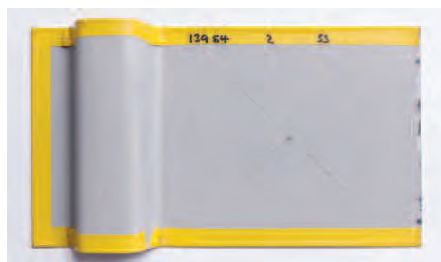
Figure 21. Test panel after humidity 1000 hours
