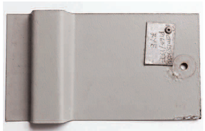
Figure 18. Colorcoat HP200® 18 years exposure at coastal weathering site at Rye, England.
