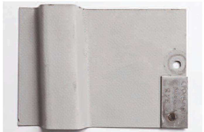
Figure 17. Colorcoat HPS200® with Galvalloy® metallic coating – 13 years exposure at coastal weathering site at Rye, England.
