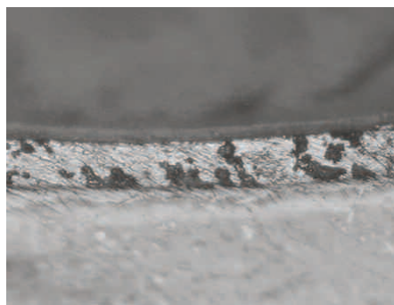
Figure 9. Galvalloy® microstructure after corrosion
