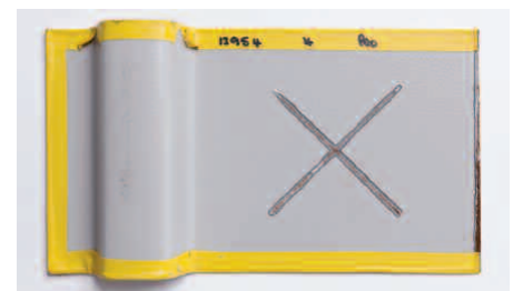
Figure 22. Test panel after Watersoak 1000 hours
