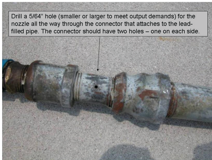
Figure 3. The nozzle for herbicide discharge can be drilled to any appropriate size. Note that the leading edges of the fitting are ground down to minimize snagging on submersed weeds. Credits: Greg Reynolds.
