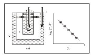
Set Up: A double walled vessel (v) containing water in between two walls.
