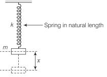
Suppose x is the maximum extension in the spring when it reaches the lowest point in oscillation.
