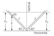
Let us consider an infinitesimal liquid column of length dx at a height x from the horizontal line.
