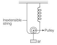
Now, if the mass is given a further displacement downwards by an amount x. The string and spring both should increase in length by x.
