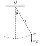
The bob is displaced through an angle  $\theta$  shown. The restoring torque about the fixed point *O* is  $\tau = -mg\sin\theta$ If  $\theta$  is small angle in radians, then  $\sin\theta \approx \theta$   $\Rightarrow \qquad \tau \approx -mg \ \theta \Rightarrow \tau \propto (-\theta)$ Hence, motion of a simple pendulum is SHM for small angle of oscillations.
