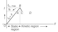
The frictional force *f* is shown on vertical axis and the applied force *F* is shown on the horizontal axis. The portion *OA* of graph represents static friction which is self adjusting. In this portion, f = F.
